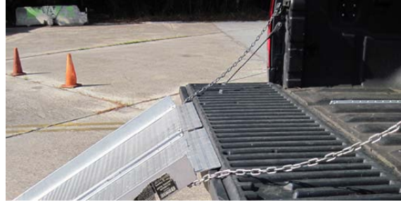
Incorrect – Chains too loose
